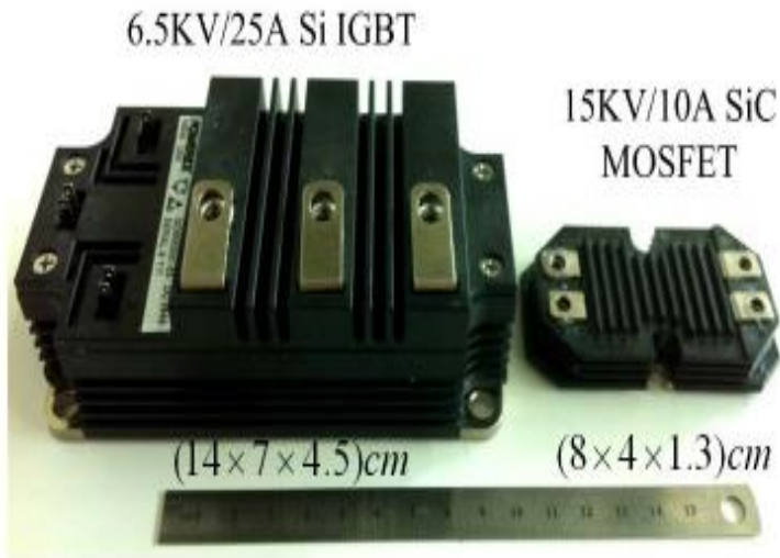
Fig 4 Size comparison between Si IGBT and WBG MOSFET.[7]
